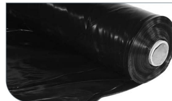
WSF 40 Optional item if non root-resistant waterproofing used Width: 8 m Length: 25 m Weight: ~ 320 g/m² 1,5 m of overlapping is necessary Sipariş Kodu: 04160001040
