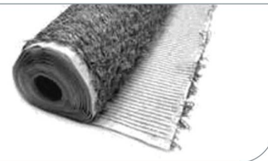
WICKING MAT DV 40 Width: 2,10 m (10 cm bini payı) Length: 25 m Weight: 600 g/m 2 Height: 40 mm (lifler dahil)
