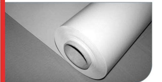
WSB 100-PO Optional item if non root-resistant waterproofing used Width: 2,44 m Length: 30,50 m Weight: ~ 1,13 kg/m² 10 cm of overlapping is necessary Sipariş Kodu: 04160001084
